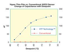
this change is quasi linear and its sensitivity to temperature is negligible. The advantages of a linear high capacitance response are: better sensitivity, better repeatability and
