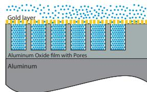
The operating principle of the HTF™ aluminum oxide sensors is that a hygroscopic layer of aluminum oxide adsorbs or releases water molecules within its pores, depending on the water vapor pressure in its environment. The electrical capacitance of the aluminum oxide layer changes with the surrounding water vapor pressure. The electrical capacitance is measured between the aluminum core of the sensor and a porous conductive gold layer on the outside.
