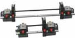
A variety of clamping fixtures are available to simplify attaching the transducers to the pipe. Transducers are integrated into the small pipe transducers up to 2" lines. For larger pipes, the transducers ship with clamps that range up to 24" pipes. For pipes up to 48", a larger pipe clamp is available with chains. If all the pipes are made from carbon steel, magnetic clamping fixtures may be the best option for fast setup.
