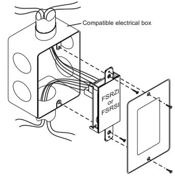
The FSRSI can be installed alone or with one or more FSRZIs. The FSRSI and FSRZI-A require trim plates (ordered separately). These are available in one, two or three gang models. Each panel will support two FSRZIs.
