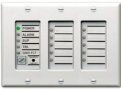
The E-FSC family has several remote annunciation options. The serial remote annunciator bus can be run up to 1000 feet (305 m) on untwisted non-shielded 18-gauge cable. Serial annunciator models round out the family to provide a range of features and functions. As many as three annunciator modules may be mounted in a standard electrical box, sharing an attractive trim plate that blends with any decor.
